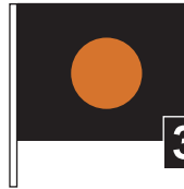
Black, Orange disc Mechanical failure
