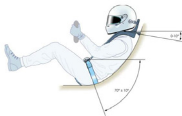
Figure 14 recommended belt angle for open cockpit cars
